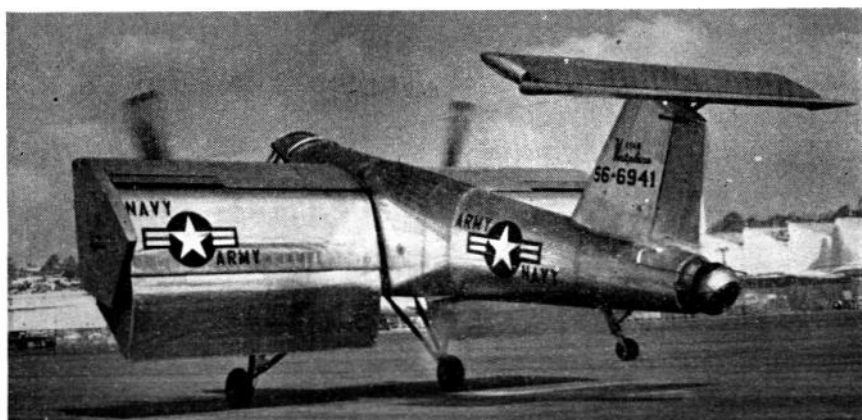
FIG. 12. RYAN model 92 Vertiplane, a deflected-slipstream research airplane.
