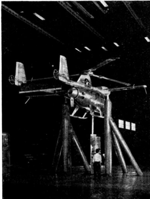
FIG. 1. McDONNELL XV-1 unloaded-rotor convertiplane in NACA Ames 40 by 80 ft. tunnel.
