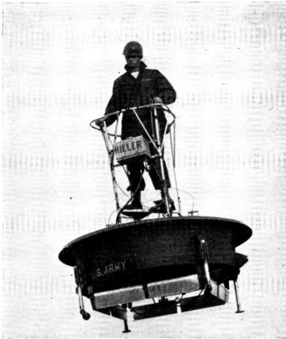
FIG. 29. Hiller ducted-fan flying platform. Original design with 5 ft dia. duct.
