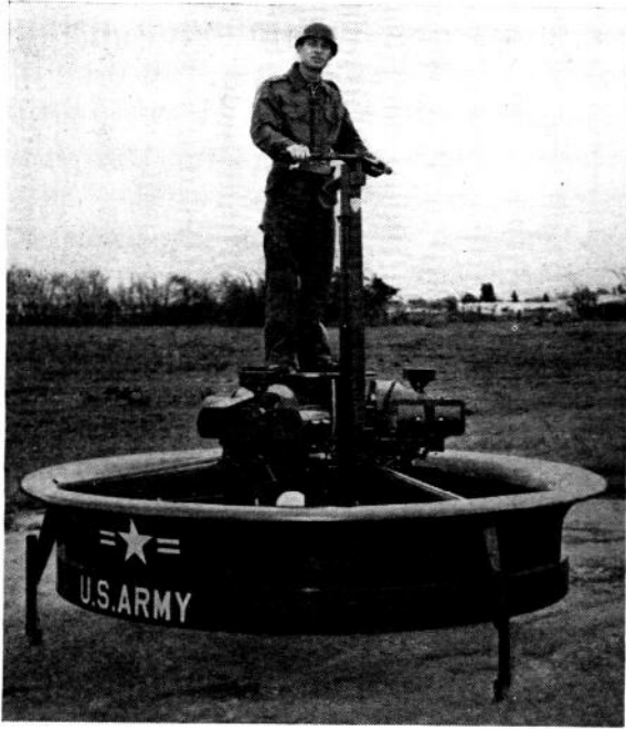
FIG. 30. Hiller ducted-fan flying platform. Revised design with 8 ft dia. duct.
