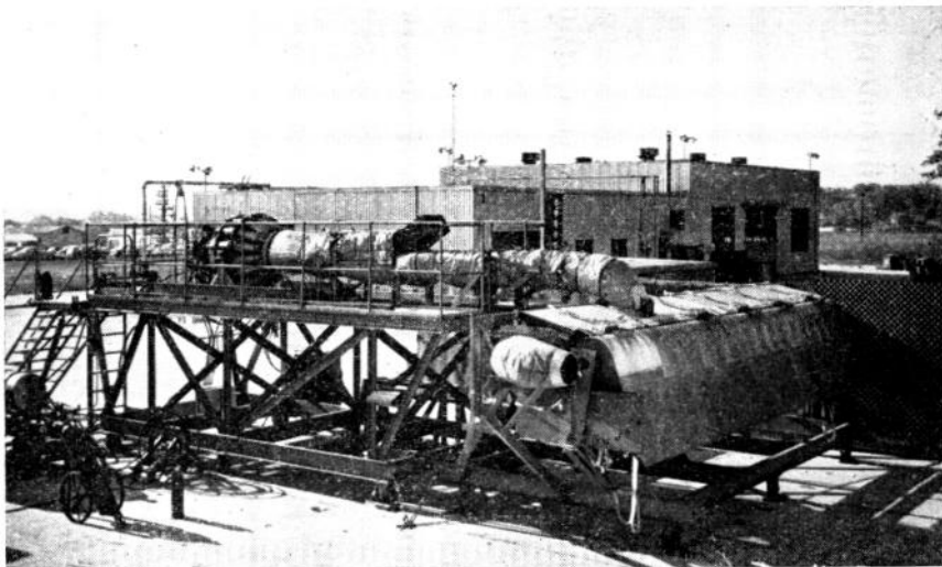
FIG. 46. Large-scale, hot-jet, static-test setup used by Martin on jet-flap studies.
