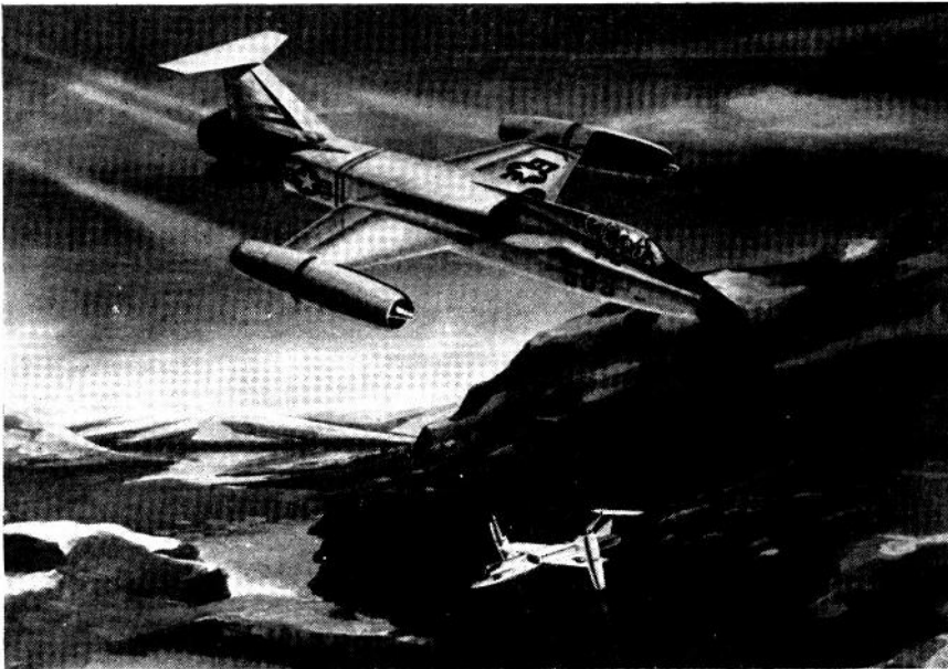
FIG. 38. Example of jet VTOL fighter-type airplane considered in studies by Bell.
