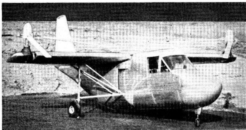
FIG. 2. Transcendental model 2 tilting-rotor convertiplane.
